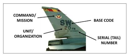
Aircraft Tail Markings. While similar, each branch of the military has unique aircraft in their inventory and their codes may vary slightly. Attachment 2, Aircraft Tail Markings, provides a generalized foundation for aircraft identifiers.
